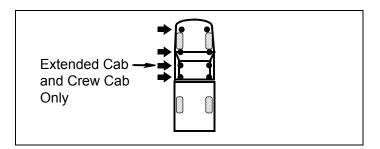
2. Remove cab mounting bolts from passenger side only. The large factory washer at the core support will be reused. Cut off bolt head and remove washer. Drill out washer to 1/2".
