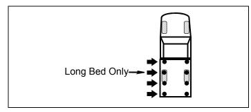
12. Remove bed mounting bolts from passenger side only.
