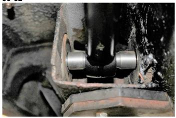
8. The 60-62 years use a 9/16" bolt, it will be reused to attached the lower bars. The Front Lower uses the WIDE(70013768) R-Joint Spacers inserted into each side of the R-Joint.
