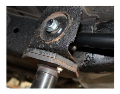
9. With the R-Joint spacers installed, hold the front of the lower bar in the factory leaf spring mount and reinstall the OEM Bolt setup.
