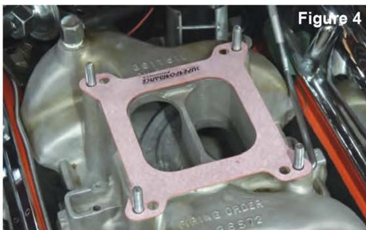
1. Place the supplied gasket on the manifold (see above) and place the throttle body onto the gasket over the existing studs. The throttle body linkage must be on the driver's side of the engine.
