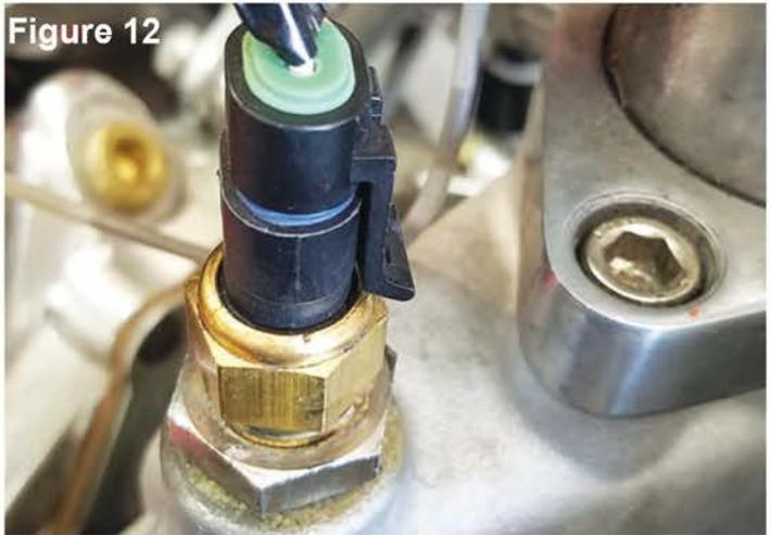
**Above** - The CTS connector on the main wiring harness is plugged into the Coolant Temperature Sensor in the manifold. (1/2" NPT adapter supplied in kit)
