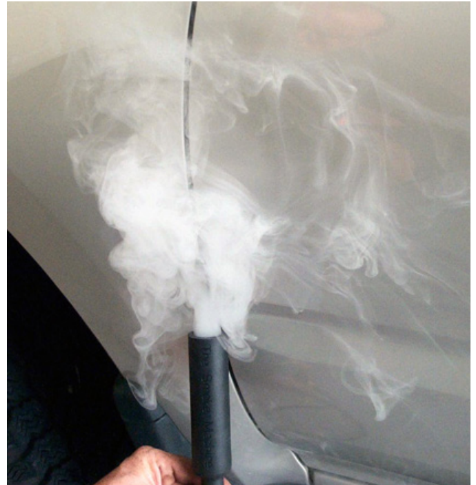
No vapor disturbance indicates no leak.
