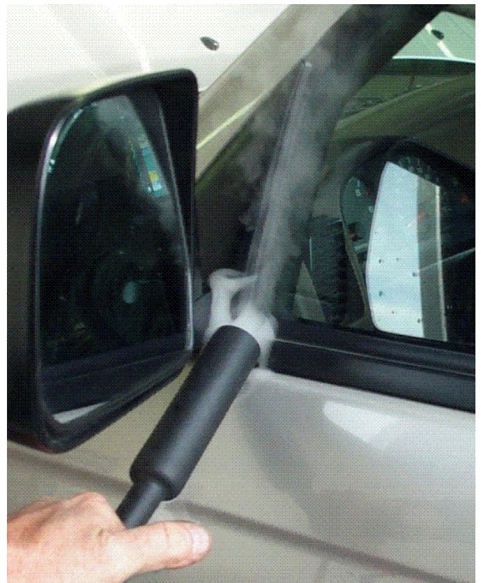
Vapor disturbance pinpoints leak.
