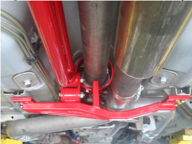
Image 3- Item # 2203 Installed with Front Drive Shaft Loop
