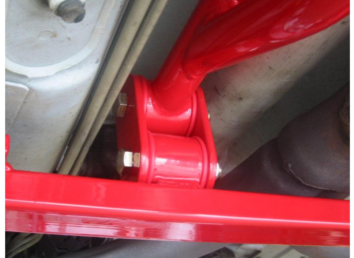
Image 2- Torque Arm Attached using Pivot Plates
