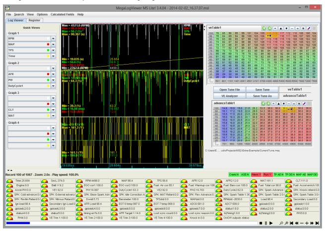
From this screen you can review many of the sensor outputs and other readings from your Megasquirt. The "Quick View" graphs are especially useful and are easily customized using the options on the left hand side of the screen.
