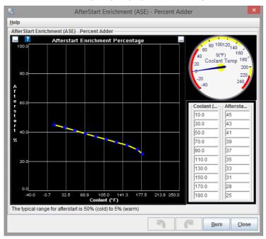
Immediately after the engine has started it is normal to need additional fuel. This curve specifies how much fuel is added as a percentage – usually (5 to 50%)
