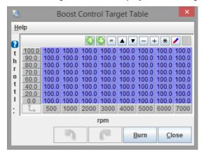
For Closed-loop boost, this table sets the target boost vs. TPS/RPM
