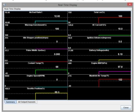
This screen shows real-time information for many of the key sensors for your Megasquirt. For further detail click the "All Output Channels" tab at at the bottom left to display a full list of variables, as shown below:
