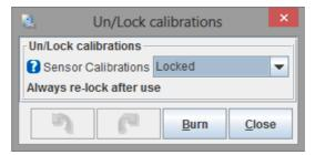
Selecting "Locked" or "Unlocked" will disable or enable the remaining calibration options.
