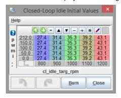
The best-guess idle valve position for RPM/load. This allows you to 'kick-start' the closed-loop idle by setting the valve to the most likely position.
