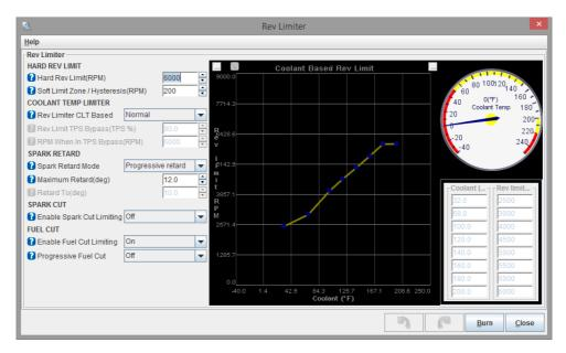
From this screen you are able to control settings such as hard rev limit, coolant temperature limit, spark retard, spark cut and fuel cut.
