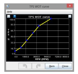
This curve sets the TPS% that is considered wide-open-throttle based on RPM.
