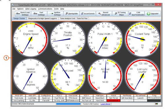
Right-clicking on any gauge in this gauge cluster will bring up a pop-up menu allowing you to swap the gauge for one of the alternatives as described in Sections 17.1, to 17.8, below:
