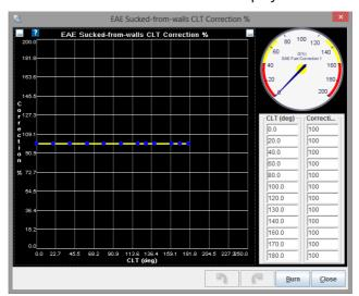
This curve modifies the EAE Sucked-from-walls curve. It allows the amount of correction specified by the EAE Sucked-from-walls curve to be increased or decreased based on coolant temperature.
