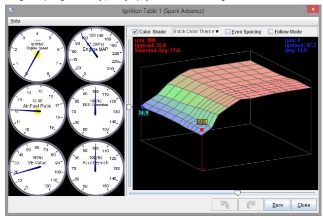
The screen will be a direct transformation of the numerical values in the matching Ignition Table. The X & Y axes represent rpm & ignition load respectively, and the height at each point reflects the degrees for the same point in the table.
