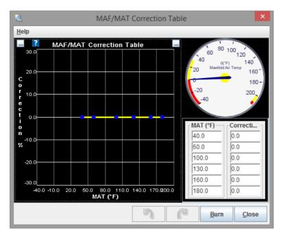
This curve allows for minor corrections to fueling based on manifold air temperature (MAT) when using MAF to control fueling. The default curve is 0% meaning no correction.
