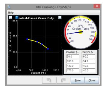
This curve sets the idle valve position during cranking. This should be set high enough so that the engine can start without touching the throttle when cold, but not so high that the engine revs up too far immediately after starting.
