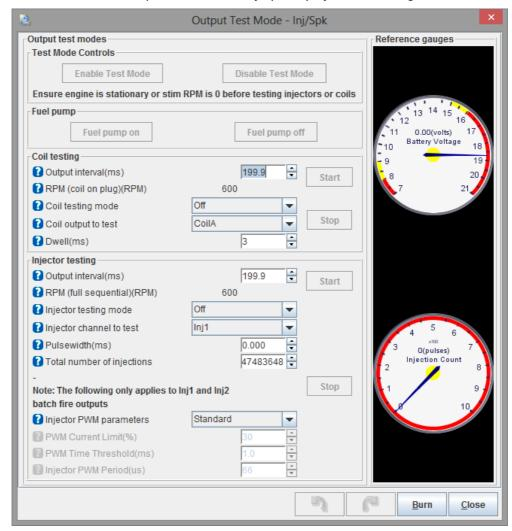
This test mode allows direct control and testing of the coils and injectors.
