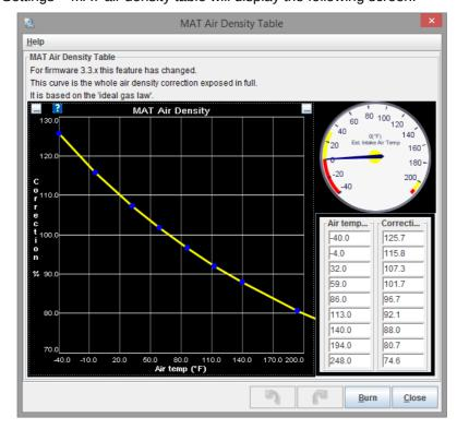
This curve is the whole air density correction exposed in full. It is based on the 'ideal gas law' and typically varies between 125% cold to 75% hot.
