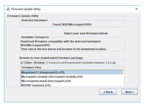
On this screen it is very important to ensure you have selected the firmware variant that matches your actual ECU. TunerStudio will try to figure this out and recommend the correct one, but you MUST check it is correct!
