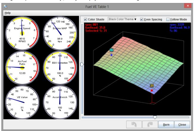
The screen will be a direct transformation of the numerical values in the matching Fuel VE Table. The X & Y axes represent rpm & fuelload respectively, and the height at each point reflects the percentage for the same point in the table.
