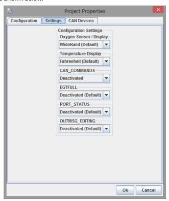
As discussed in Section 2.1.1. the contents of this tab will depend on the version of the firmware that you are using. The default settings should be expected to work with your Megasquirt, but they can be changed at any time as required.
