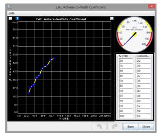
This curve determines how much fuel is being added to the port walls per injection event. It is a percentage (Y-axis) of each injection event based on load (X-axis).
