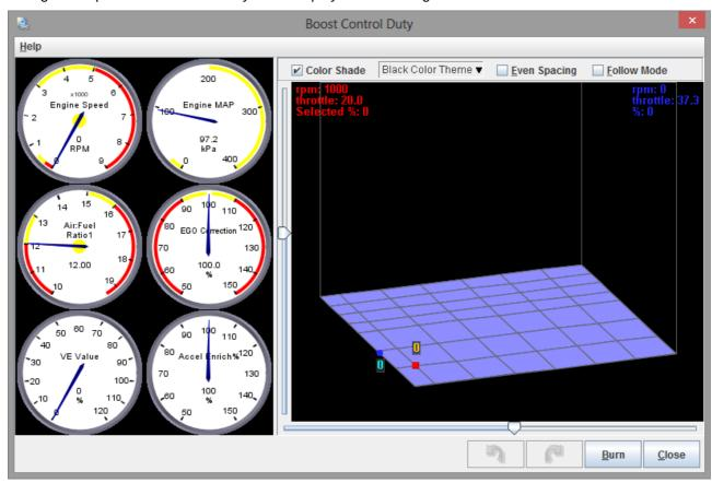
The screen will be a direct transformation of the numerical values in the Boost Control Duty Table. The X & Y axes represent rpm & throttle respectively, and the height at each point reflects the percentage for the same point in the table.
