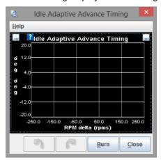
Sets the timing vs engine load when Idle Advance is active. Typically the curve will ramp from higher advance at negative RPM deltas (below target) to lower advance at positive RPM deltas (above target) to help stablise idle.
