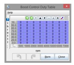
For Open-loop boost, this table sets the output duty cycle vs. TPS/RPM.
