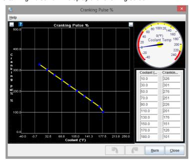
This percentage table controls the fuel injected when the engine is cranking. Most engines need 200-400% when cold and near 100% when hot.
