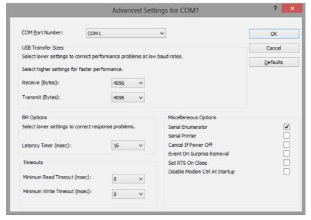
Using this screen you can change the COM Port Number for the port connected to your Megasquirt. If you want to use COM1 and another device is already using COM1, you will need to change the settings for that other device before setting up the port for your Megasquirt. The Latency Timer should be set to the minimum value (1).
