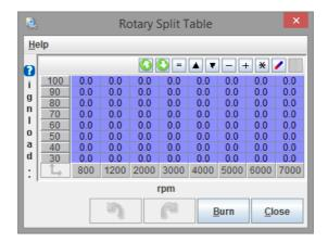
This table specifies the split (delay) in degrees between leading and trailing coils.
