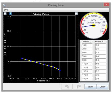
The priming pulse is used to wet the intake manifold walls and provide some initial starting fuel.
