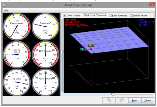
The screen will be a direct transformation of the numerical values in the Boost Control Target Table. The X & Y axes represent rpm & throttle respectively, and the height at each point reflects the percentage for the same point in the table.
