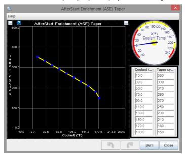
Specifies how long (in engine cycles) to apply afterstart enrichment.
