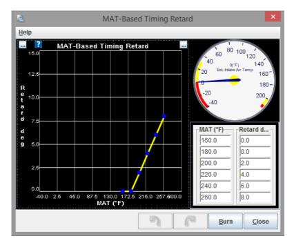
This curve allows ignition timing to be retarded based on intake temperature. This is primarily for forced induction installs where there is charge heating.
