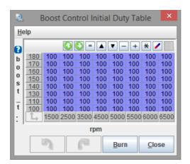
The best-estimate boost valve duty for target load vs. RPM. This allows you to 'kick-start' the closed-loop boost by setting the valve to the this position before engaging closed-loop PID control.
