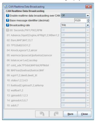
Once enabled, the user can select which data packets to broadcast and at what frequency. Be aware that the maximum capacity of CAN is around 4000 packets per second i.e. 40 channels at 100Hz. For reliable operation of other devices on the network it is suggested that a lower limit of 1-2000 be applied.
