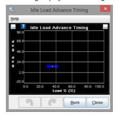
Sets the timing vs. engine load when Idle-Advance is active. Typically the curve will ramp from low advance at low load to more advance at higher loads to stabilize idle.
