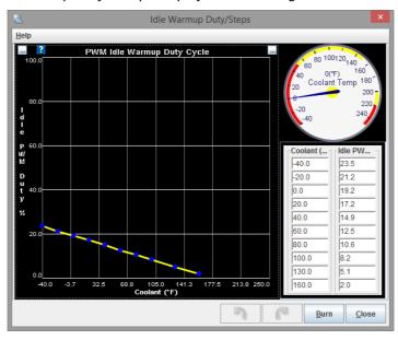
This curve specifies the PWM Idle Duty vs. coolant temperature to be used during warmup.
