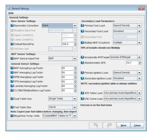
From this screen you can set values for many of the settings you may need for your configuration, including barometric settings, MAP sensor settings, general sensor settings and secondary load parameters.
