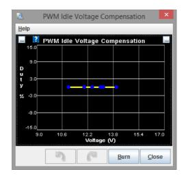
Some 2 wire PWM idle valves will operate differently depending on the system voltage. This allows a compensation to be applied to allow for that difference.
