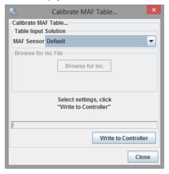
From this screen you can set the MAF (mass air flow) calibration if needed. The options for these settings are described below:
