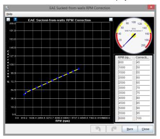
This curve modifies the EAE Sucked-from-walls curve. It allows the amount of correction specified by the EAE Sucked-from-walls curve to be increased or decreased based on RPM.
