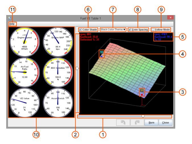
Whilst 3D Maps can appear quite complex at first glance they are actually relatively simple. For each of the 256 points in the 3D table, a 3D map is created using the X and Y axis, with the height at each point reflecting the numerical value (often referred to as the Z axis). This allows you to get a feel for the gradients within your tune. Like 3D tables, lower numbers are shown in blue and higher numbers are shown in red with green representing mid-range values.
