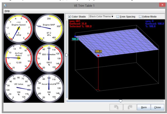
The screen will be a direct transformation of the numerical values in the matching Fuel VE Trim Table. The X & Y axes represent rpm & fuelload respectively, and the height at each point reflects the percentage for the same point in the table.
