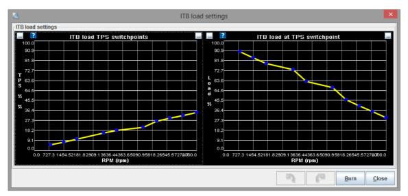
The left hand curve defines the TPS value where the MAP load reaches %Baro switchpoint. This curve will be different for each engine and should be set up using values obtained from log files from your engine. Setting this curve is an important part of ITB mode.
