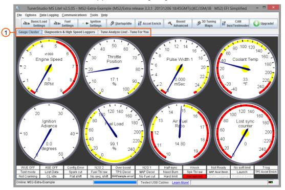
"Gauge Cluster" is the default tab which is displayed when you open TunerStudio. Using the default dash this gives you access to eight customizable gauges and a set of indicators. The gauges are labeled as (1) in the following image and are documented in this section. The dash indicators are documented in Section 18.
