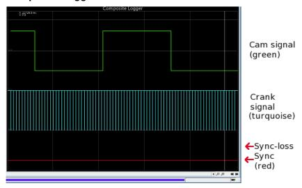
This logger records both crank and cam signals in a format similar to an oscilloscope. The exact display will depend on a number of factors
