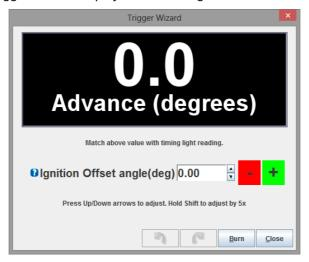
In 'Basic Trigger' and 'Trigger Return' this specifies the engine angle BTDC that each trigger pulse is received.
