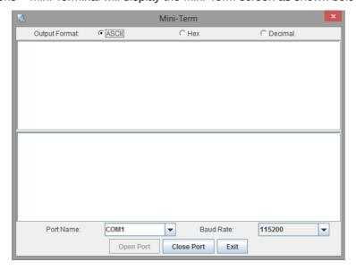
As simple example of how Mini Terminal works is as follows: With your MS2 connected and powered up, typing "S" into the top half of the screen should display the version of your Megasquirt and the firmware that it contains as shown below:
