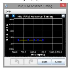
Sets the timing vs engine RPM when Idle Advance is active. Typically the curve will ramp from higher advance at lower RPMs to less advance at higher RPMs to stablise idle
