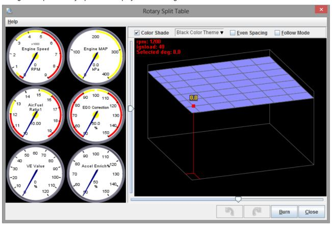
The screen will be a direct transformation of the numerical values in the Rotary Split Table. The X & Y axes represent rpm & ignition load respectively, and the height at each point reflects the degrees for the same point in the table.
