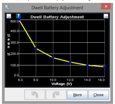
This curve specifies the percentage adjustment to the nominal dwell based on battery voltage.
