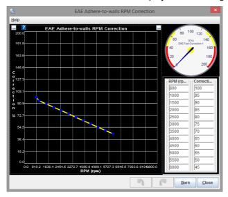
This curve modifies the EAE Adhere-to-walls curve. It allows the amount of correction specified by the EAE Adhere-to-walls curve to be increased or decreased based on RPM.
