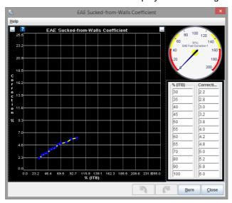
This curve determines how much fuel is being sucked from the walls on each intake (valve open) event. It is a percentage (Y-axis) of the total amount of fuel that has adhered to the walls based on load (X-axis), so therefore the percentages are much smaller (about 10x smaller) than the Adhere-to-walls coefficients.
