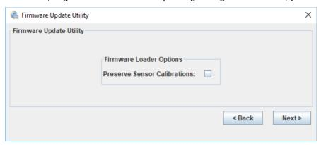
In this example, we are loading firmware to a fresh 'blank' processor, so be sure NOT to Preserve Sensor Calibrations as there is nothing to preserve.
