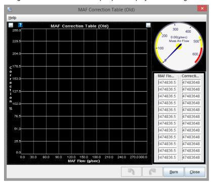
Specifies the adjustment on top of the MAF sensor calibration you loaded through Tools-Calibrate MAF table. Start out with the correction curve at 100% (no correction) and then 'tweak' to tune it to your install.
