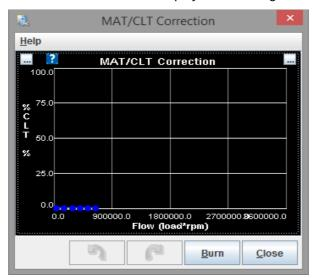
The curve is the %CLT blended into the MAT reading vs. airflow.
