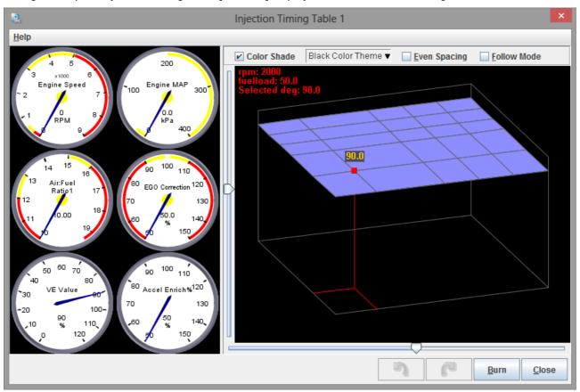
The screen will be a direct transformation of the numerical values in the matching Injection Timing Table. The X & Y axes represent rpm & fuelload respectively, and the height at each point reflects the degrees for the same point in the table.
