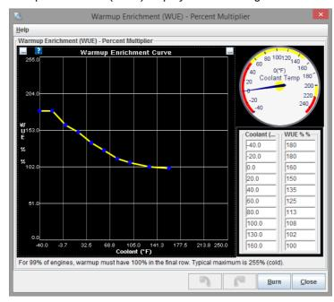
Specifies the percentage multiplier for fuel during warmup. At cold temperatures 200-300% may be required.
