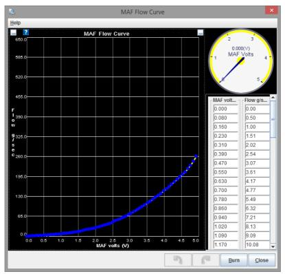
This curve specifies grammes/sec versus voltage. Start out with the actual flow curve for your MAF sensor and then 'tweak' to tune it to your install.
