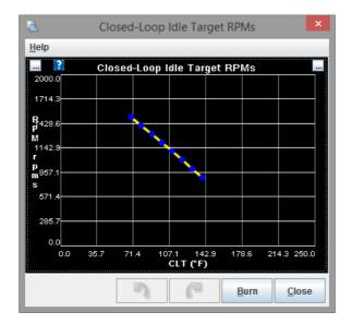
This curve displays the closed loop idle RPM target depending on coolant temperature. It is normal to set a high idle on a cold engine, tapering down as the engine warms up.
