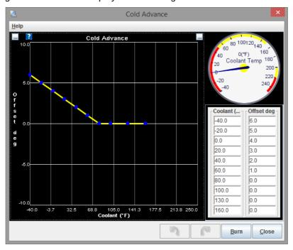
This curve optionally allows ignition timing to be advanced during warmup. Conversely, some engines may prefer retard during warmup (to pre-heat the catalytic convertor).
