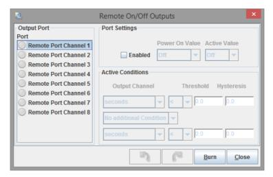
This screen will be familiar from Section 13.10 which covers the built-in programmable On/Of Outputs. The main difference is that an expansion card will give additional remote On/Off outputs in addition to those which are built into your Megasquirt. The documentation that shipped with your expansion card will be necessary to configure these outputs accurately, although the basic concepts are the same and are described below.
