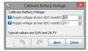
These settings can be used to correct battery voltage readings at (and between) zero and max.
