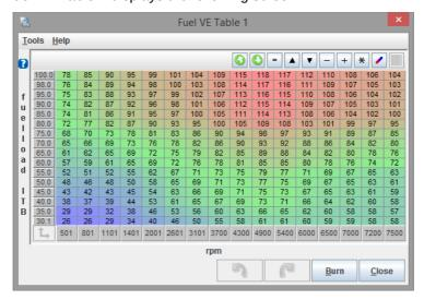
This is the main fuel table [VE1]. Fuel VE table size can be set to either  $12 \times 12$  or  $16 \times 16$  – this option can be set through Basic/Load Setting > General Settings (see Section 8.2.3.)
