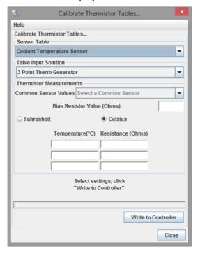
From this screen you can set the CLT (coolant temperature) calibration if needed. The options for these settings are described below:
