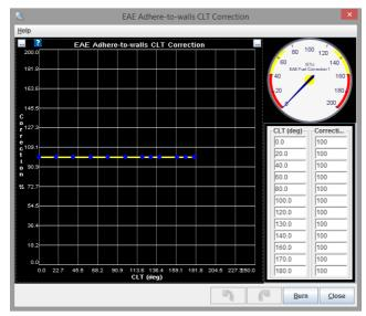
This curve modifies the EAE Adhere-to-walls curve. It allows the amount of correction specified by the EAE Adhere-to-walls curve to be increased or decreased based on coolant temperature.
