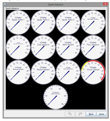
This screen is for information purposes only and displays the spark advance at any given stage when the engine is running. This screen can be useful for analysis and troubleshooting.
