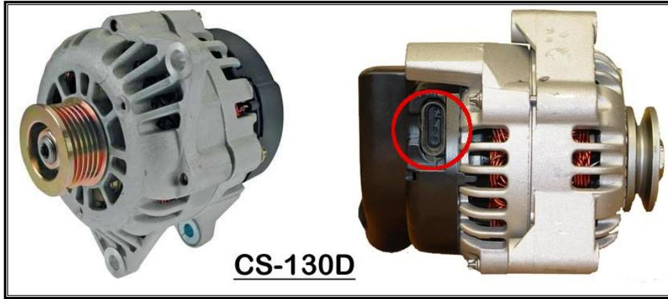
The CS-130D can be spotted by the lack of an external fan behind the pulley. These alternators have an internal fan and a plastic casing on the back. These alternators have an elongated, oval, 4-pin, sealed connector, seen circled in the image above. The regulator will be marked P, L, I, S. This type of alternator was used on many engines, including the GM LS series, Vortec, and Gen. III Vortec truck fuel injected engines.
