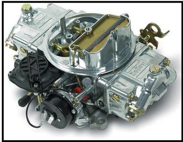
When you turn your key to the “ON/RUN” position, the voltage this wire carries heats the bi-metal spring called the “choke thermostat.” This spring will unravel as it is heated causing the choke to slowly open. When the ignition is turned to the “OFF” position, power is no longer on this wire, causing the spring to begin to cool and contract, closing the choke.
