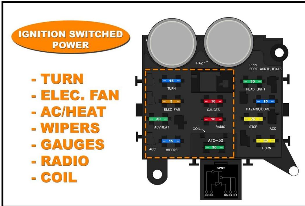
The drawings on this page show all the switched ignition fuses. These fuses are powered by wires coming from the ignition switch (wires #931, #932, and #933) and receive power depending on what position the ignition switch is in. **NONE OF THESE FUSES SHOULD HAVE POWER WHEN THE IGNITION IS IN THE OFF POSITION.** The **Ignition Switch Section** beginning on [page 68](#) of this manual will go into further detail about power supplied to these fuses.
