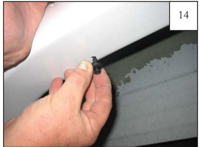
Position flare on vehicle and reinstall Retainers (RV1-P001) .
