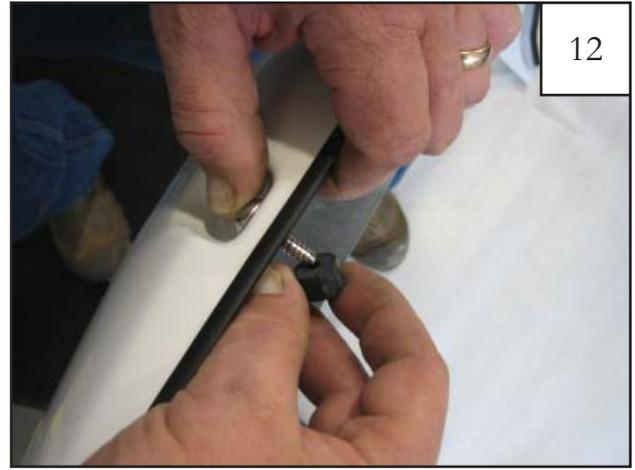
Install a supplied Screw (SW1-0045) through each pocket hole in flare and thread a Spacer (SP1-0009) over the end.
