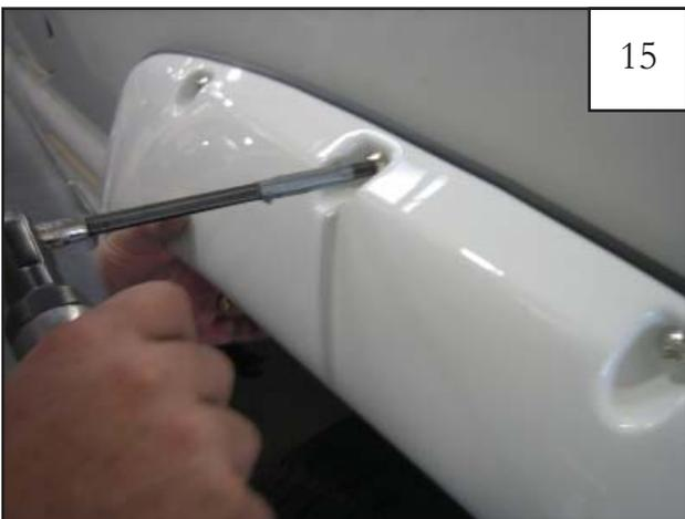
Using the supplied Torx Bit (SW1-0052), install Screws (SW1-0045) through 3/16" holes drilled in Step 11. *Do not overtighten Screws. Overtightening will not allow the flare to expand and contract with temperature changes after installation and may deform the part.*
