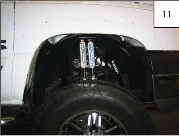
Remove the flare. Using a 3/16" drill bit, drill through the marks made in previous step.
