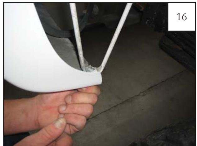
Reinstall factory support rod bolts through the 3/8" holes in flare and secure, making sure not to overtighten and crush flare.
