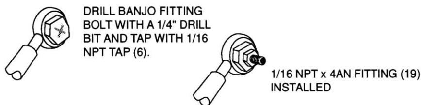
Figure 13 Schematic of “Drilled Out” Banjo Fitting
