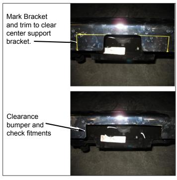
e. Install rear bumper onto *kit* **bracket** (rear bumper, middle) with two *kit* **bolts** (7/16" x 1-1/4"), four *kit* **washers** (7/16" USS) and two *kit* **nuts** (7/16" Nylock). DO NOT TIGHTEN.
