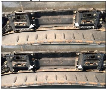
b. Place kit front bumper bracket over driver frame horn, clamp it in place. Mark and drill two 1/2" holes "centered" where marks are shown (Be sure that everything is centered before drilling) Repeat steps to passenger side.
