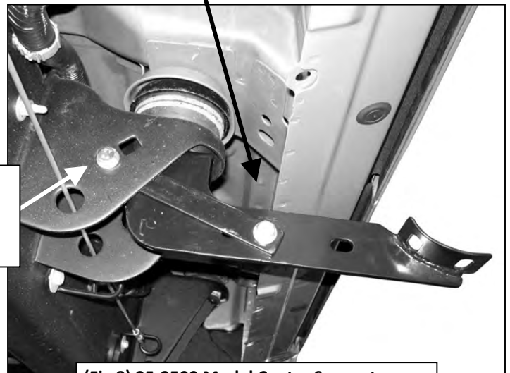
(Fig 8) 25-3500 Model Center Support Bracket Installation Pictured
