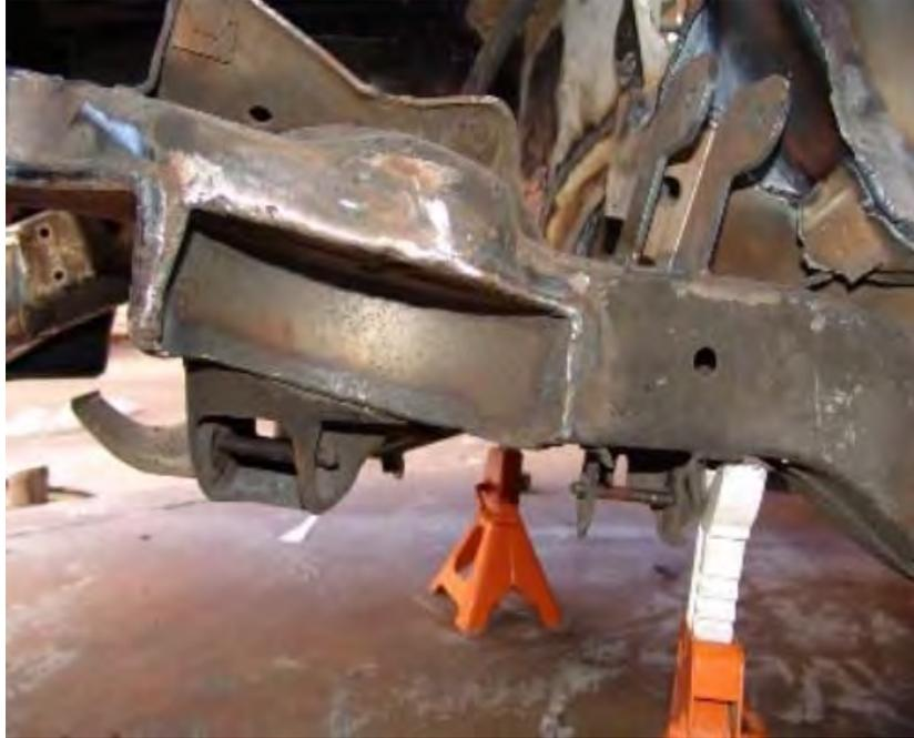
Driver side with control arms and spindles removed.
