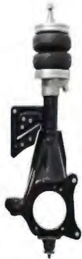
**We do not sell a universal kit. Our struts are built EXACTLY to Original Equipment Specifications. In most cases, you simply remove your factory strut and install the Airstrut. We include a Schrader manual fill valve so you can test the travel and ride height before you hook up your Plug & Play air Management System.**
