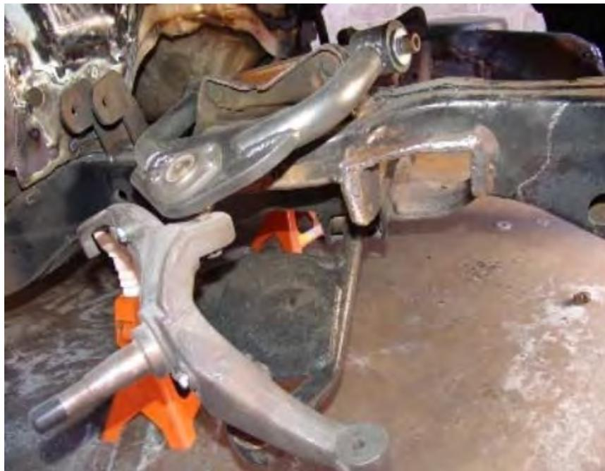
Passenger side with control arms installed and spindle turned to the right.
