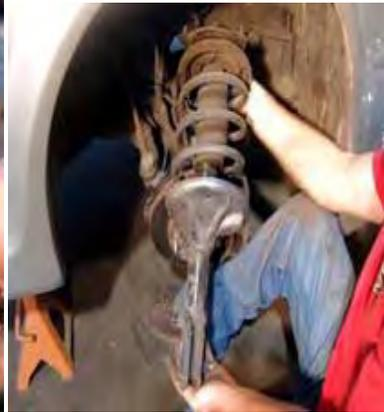
**Remove Factory Strut. In most cases, you will reinstall the top bearing plates shown below.**
