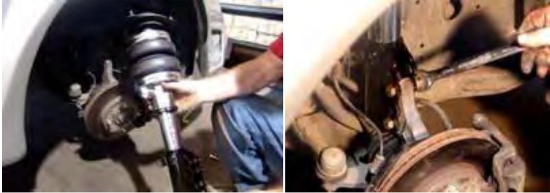
On many of our struts, you might find an extra set of mounting holes on the bottom Clevis. For the lowest position, select the top holes.
