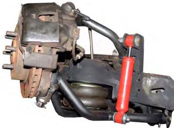
If you are not UPGRADING to the Eliminators, you will install the standard Barrels at this point.
