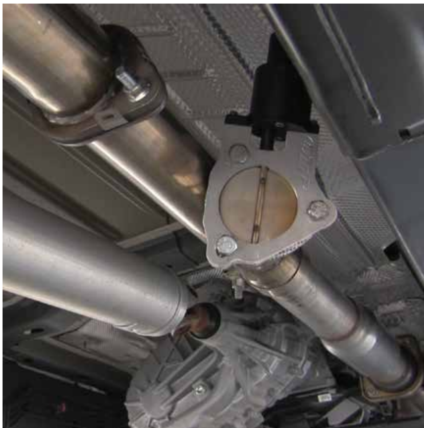
Image C: QTEC Valved installed on Aggressor Pipe
