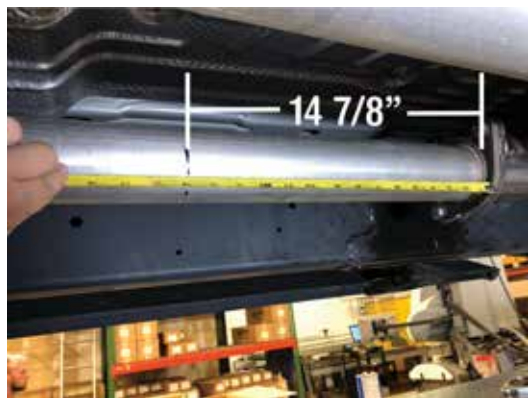
Image A: Cut Location, 14 7/8" from flange
