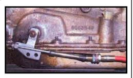
onto the threaded end of the cable and turn it until it lines up with the forward hole of the shift lever. Install the cotter pin. If it needs more travel, loosen the large nuts and washers and move the cable forward or backward to gain more travel. Then retighten the large nuts and washers. Install the small nut and tighten.
