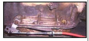
the large washer, nut and two boots. Rotate the shift lever clockwise to the park position. Now you are going to put the swivel onto the threaded end of the cable and turn it until it lines up with the middle hole of the shift lever. Install the cotter pin. If it needs more travel, loosen the large nuts and washers and move the cable forward or backward to gain more travel. Then retighten the large nuts and washers. Install the small nut and tighten.
