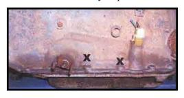
10. The two transmission pan bolts could be either Metric or American threads. You will need to purchase two bolts 1/4" longer than the two that you removed. Spacers need
