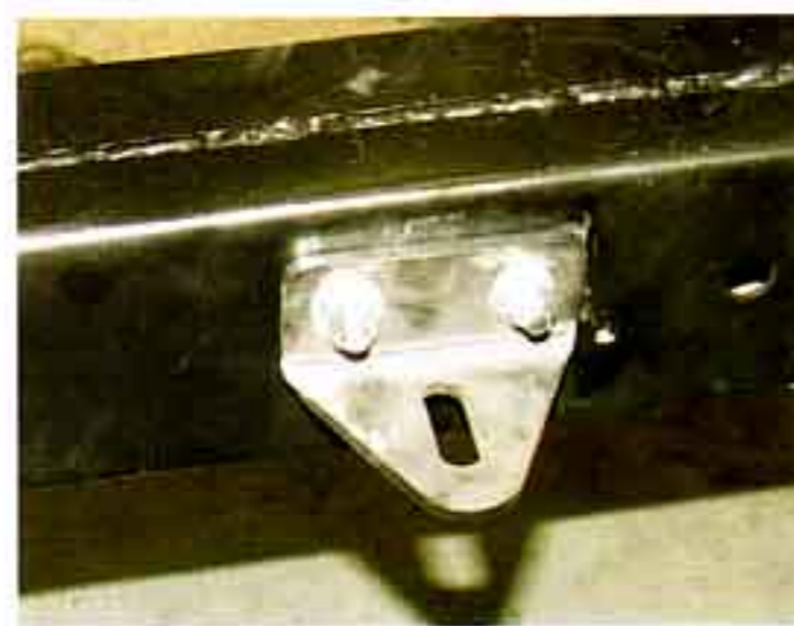
Photo #16a & 16b: The elbow mounting brackets and outer backing plates are held to the frame with two 3/8" X 5" bolts with flat washers, lock washers and nuts.
