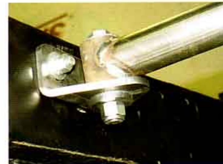
Photo #17a & 17b: Now reinstall the transmission crossmember and bolt the crossmember to the elbow brackets and transmission mount.
