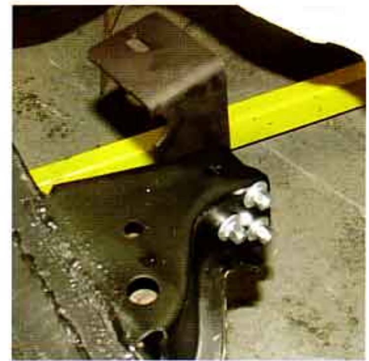
Photo #6a & 6b: The lower half of the new transmission supports bolt to the front of the original frame horns with three 3/8" X 3-1/4" bolts, flat washers, lock washers and nuts. There is a cut-out on the drivers side lower bracket to allow the front emergency brake cable to pass by.
