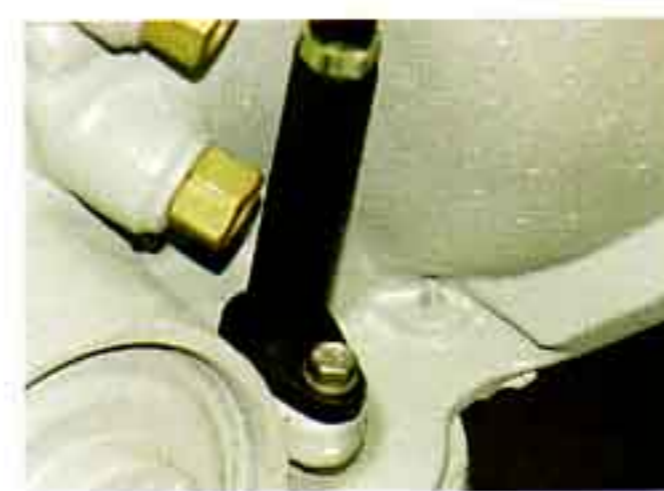
Photo #20: The TVI cable is held to the transmission case with a 10mm bolt.
