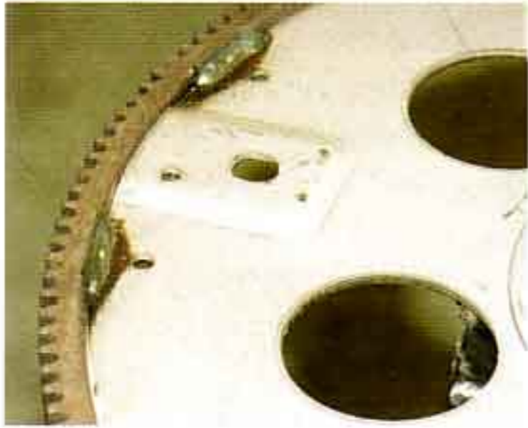
Photo #2: Begin by installing the TH flexplate on the engine. The automatic flexplate, P/N 19-30, has raised areas where the torque converter bolts on. Make sure the raised area is facing to the transmission.
