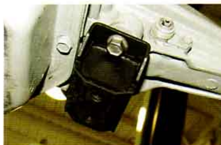
Photo #10: The transmission mount P/N 19-18 bolts to the tailshaft housing using the two 10mm X 40mm bolts supplied with the kit.
