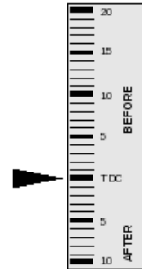
Timing marks on damper
