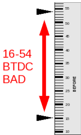
Timing marks on damper
