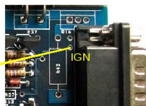
Add two 1k 1/8W resistors as shown. One on D14, one on D16
