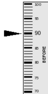
Timing marks on damper
