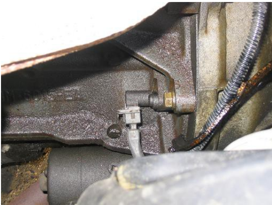
Escort / Fiesta location on engine flange above starter.
