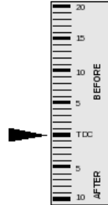
Timing marks on damper
