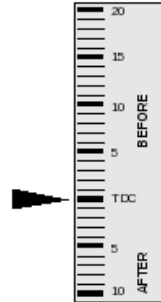
Timing marks on damper
