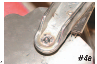
Photo #4a & 4b & 4c & 4c & 4d & 4e: With the roller and rivet in place, first use a tapered punch and flare out the tube end of the rivet. Next using a flat punch, smash the edges of the tube rivet down tight on the window frame. This will center and tighten the rivet in the hole on the window frame or regulator.
