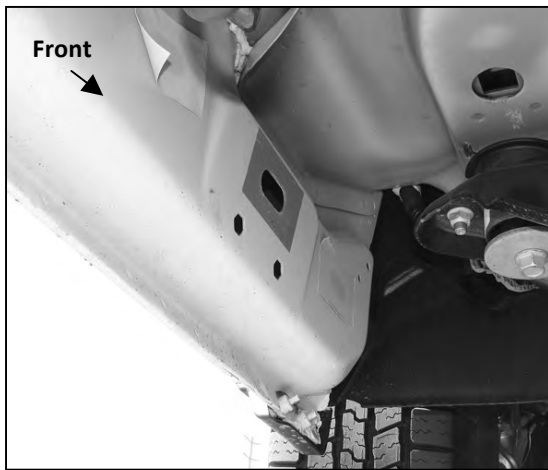
(Fig 1A) Driver/Left front mounting location
