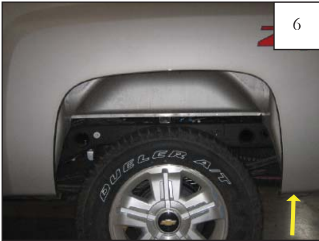
Remove one factory bolt with a 1/2" wrench.
