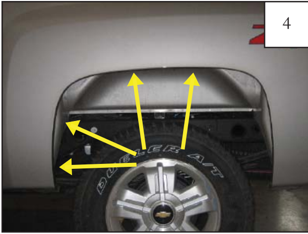
Remove four factory fasteners with a pry tool.
