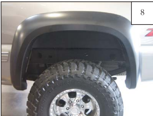
Completed rear flare installation.
