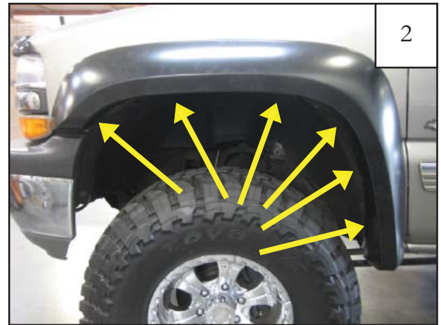
Install six tuflocks using a #2 stubby screwdriver.
