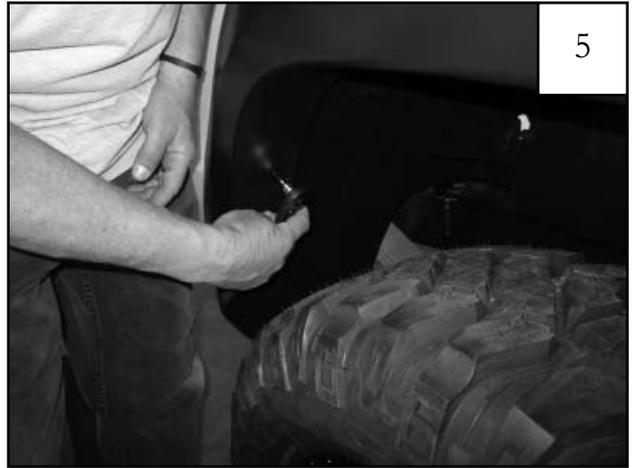
Place flare on vehicle and install one factory screw where shown to hold in place.
