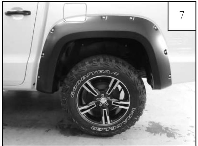
Remove flare and enlarge the marks on bumper cover.
