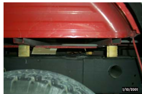
3 x 2 x 2-1/8 Overload spacers installed
