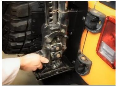
2. Insert and hold the supplied aluminum spacer between the lowest hole on the jack handle and the threaded bung in the Accessory Mount. Thread the supplied 3/8" x 2" bolt with washer through the jack handle and spacer, and into the threaded bung. Do not tighten yet.
