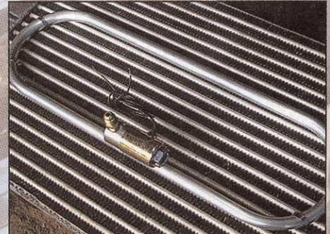
Step 3 Position spray bar and fit clips.
