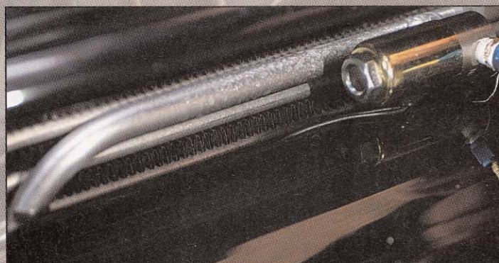
Step 1 Connect wires to solenoid and run into car.
