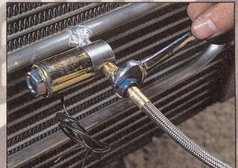
Step 6 Connect hose to solenoid.
