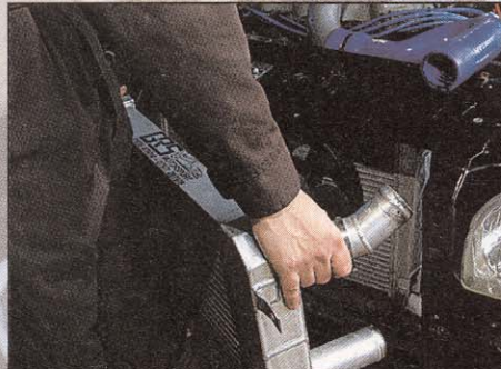
Step 2 Remove intercooler.
