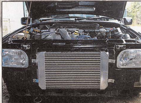
Step 1 Undo and remove front bumper.
