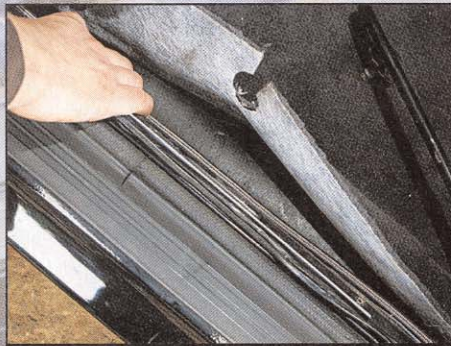
Step 2 Run hose under carpet. Drill hole in bulkhead.
