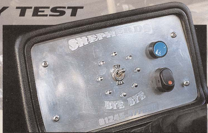
Step 4 Drill holes and fit switches.
