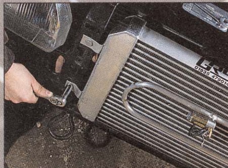
Step 5 Refit intercooler.
