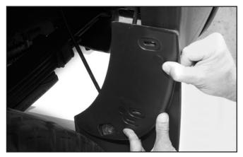
The slots in the MudFlap will line up with the holes in the fender.
