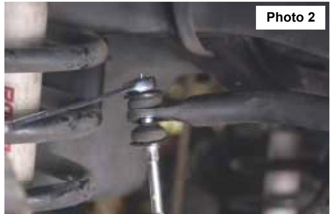
7. Remove the track bar from its upper mounting point on the frame using a 24mm wrench and rest it on the axle. It may be helpful to loosen the lower track bar bolt on the axle. Retain hardware for reuse.
