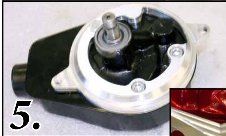
**FIG 5.** Install The Adapter Ring (21074-A) to the Power Steering Unit with (2)  $\frac{3}{8}$  x  $\frac{3}{4}$ " SHCS (S244) and (1)  $\frac{3}{8}$  x 1" Hex Bolt (S312) as Shown.
