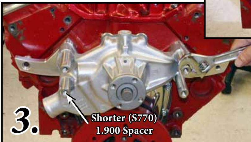
**FIG 3.** Slide the Water Pump (P112) Over the Studs and secure with the (3)  $\frac{3}{8}$ " x 2.800" Stainless Spacers (S775) two to the upper water pump studs and one to the lower drivers side water pump stud. Install (1)  $\frac{3}{8}$ " x 1.900" Stainless spacer (S770) on to the lower passenger side water pump stud. Use a sealer if necessary.
