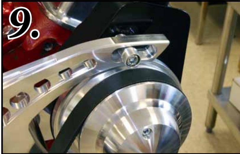
**FIG 9.** In the upper alternator adjustment slot install the provided MM100 Adjustment Bushing and the  $\frac{5}{16}$  x  $1\frac{1}{4}$ " SHCS (S148). In the Upper P/S slot use a MM100 Adjustment Bushing and a  $\frac{5}{16}$  x 1" SHCS, leave loose.
