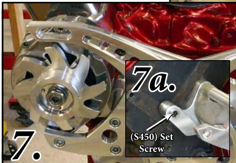
**FIG 7.** Install (S450) threaded bushing into alternator rear support bracket (as shown Fig 7a). Install the Alternators (P573) using (1)  $\frac{3}{8}$  x 5 $\frac{1}{2}$ " SHCS (S280) and a TP3-1.775 Spacer Between the rear of the Alt and the (S450) Set Screw. Turn the S450 set screw to take up any slack between the lower alternator support and the spacer. Secure with a  $\frac{3}{8}$ " Lock Nut. (S622). (snug only at this time).
