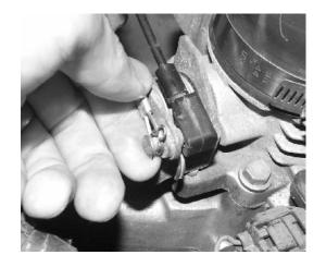
Feed the cable from the firewall through the hollow screw you had assembled onto the "L" shaped bracket earlier. Shove the end of the black rigid cable housing into the head of the hollow screw.
