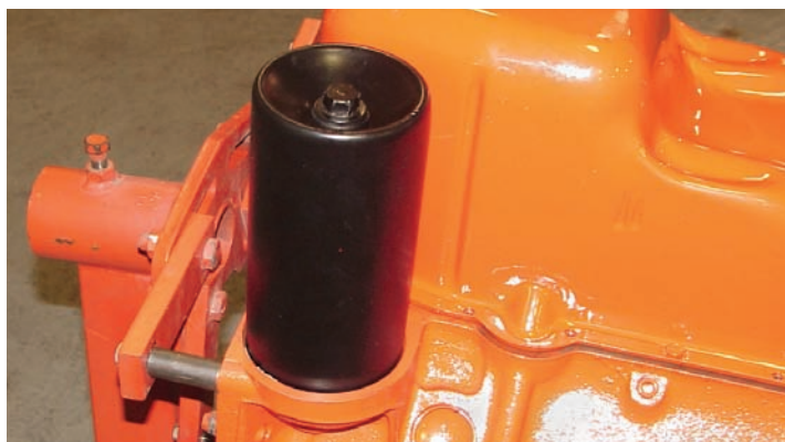
Photo #2: The oil filter canister is held to the engine block with a 3/4" right hand thread bolt in the center of the canister.
