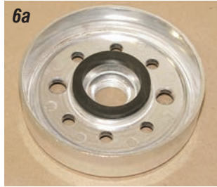
Photo #6a & 6b: The spin-on oil filter adapter P/N 18-328 (supplied with kit 18-70), mounts up in the block over the valve assembly, P/N 18-43. The outer ring of the adapter seals to the engine block using a new o-ring seal supplied with the adapter. There is a machined ring in the center of the adapter. The smaller o-ring seal supplied with the adapter should be installed here to seal against the valve assembly.
