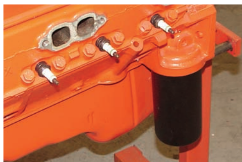
Photo #1: The oil filter assembly on small and big block Chevy engines is located at the rear of the engine next to the oil pan on the driver's side of the engine.
