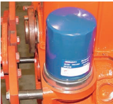
Photo #9: The new spin-on filter, P/N 18-327 (supplied with kit 18-70), will now screw onto the filter adapter and provide a clean, leak-free seal.
