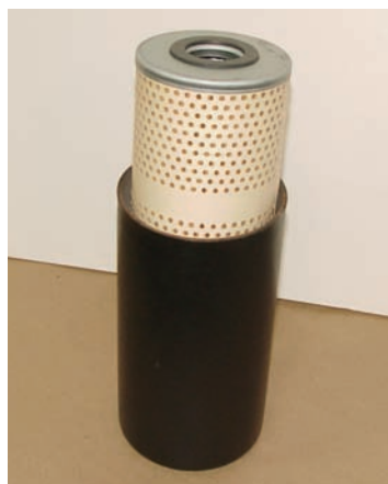
Photo #3: The original oil filter is a cartridge type filter that is installed inside the oil filter canister.
