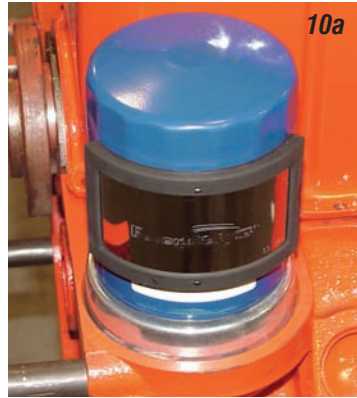
Photo #5: There is a gasket that seals the valve assembly to the engine block. This gasket must be in good shape and leak-free. If the gasket is leaking, unfiltered oil will return to the engine.
