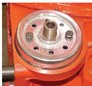
Photo #8: A 3/4" nipple and thread locker is supplied with the oil filter adapter. Place a few drops of the thread locker on one end of the 3/4" nipple and screw it into the filter adapter. Allow the thread locker to dry for one hour.
