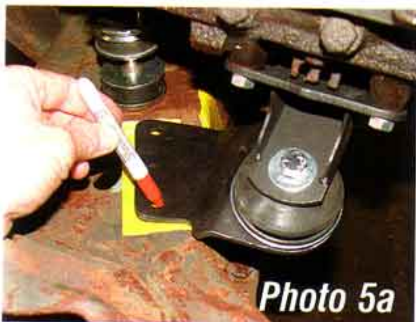
Photo #5a & 5b: Bolt the upper and lower bracket together using the 7/16" X 2-1/2" bolts and lock
