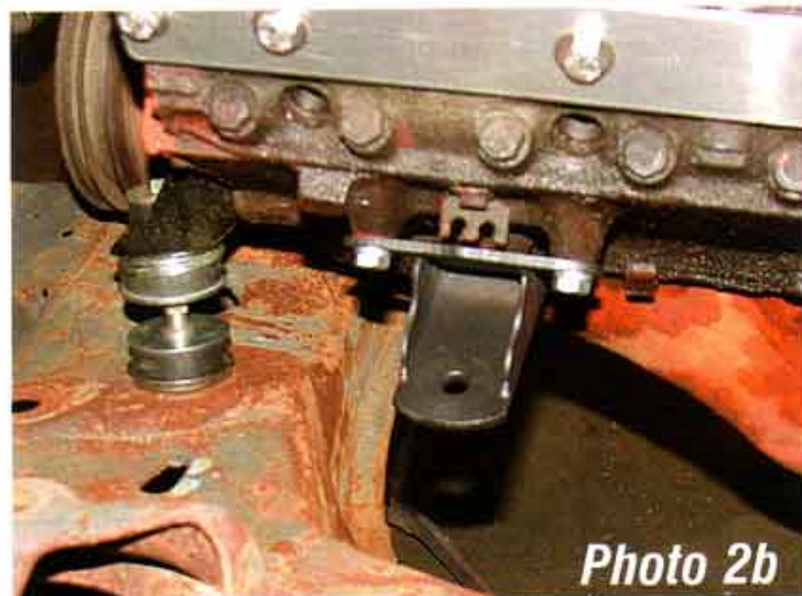
Photo #2a & 2b: The upper bracket for the side engine mount bolts to the side of the engine with three 3/8" X 1" bolts and lock washers supplied with the mounting kit.
