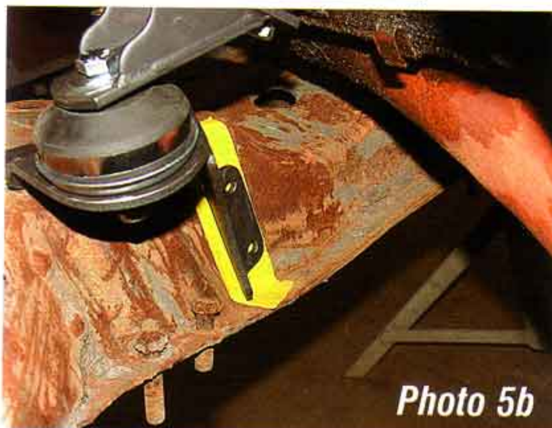
Photo #5a & 5b: Bolt the upper and lower bracket together using the 7/16" X 2-1/2" bolts and lock
