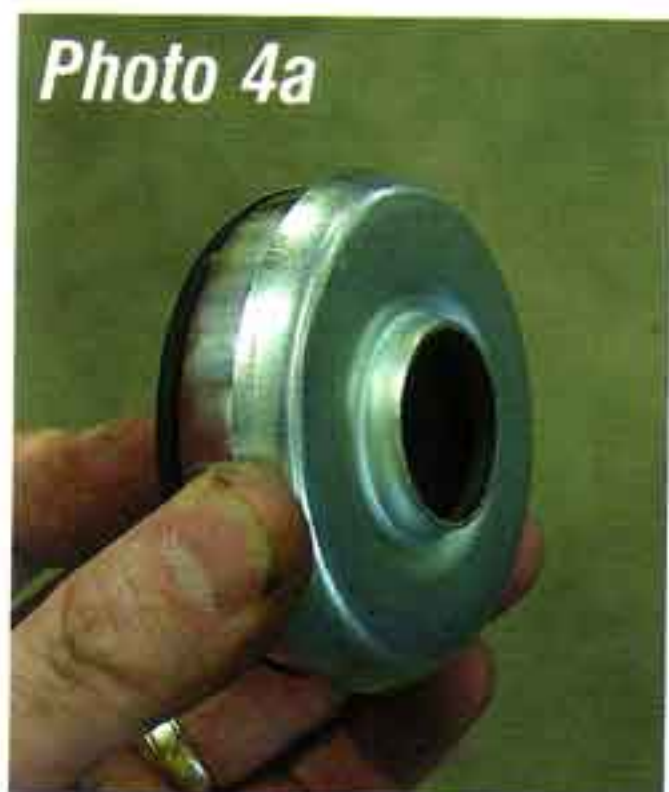
Photo #4a & 4b: The side engine mount kit uses a doughnut-style rubber mount. The lower bracket is mounted 90-degrees from the upper engine side mount bracket. The larger doughnut mount fits between the upper and lower bracket and has a steel collared washer that fits on the lower bracket. The small rubber mount fits on the bottom of the lower bracket to completely insulate the engine and any vibrations from the frame.
