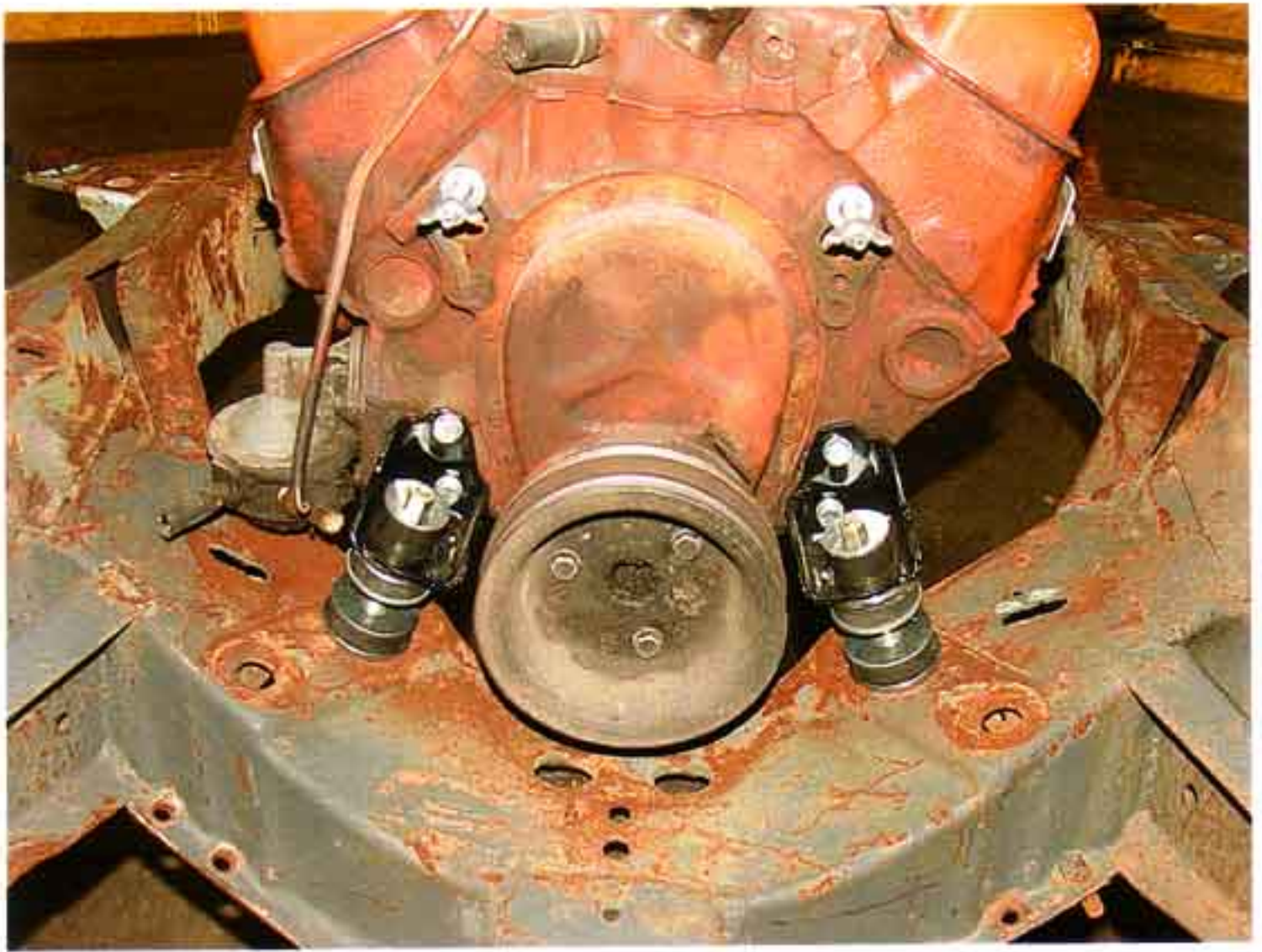
Photo #1: This shows the stock front motor mounts for a small block engine. Notice the studs are in the rear holes of the engine crossmember. The front holes are for mounting a 6-cylinder engine.
