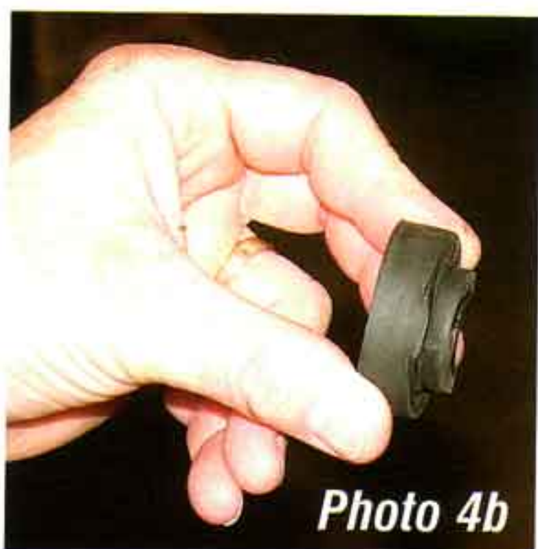
Photo #4a & 4b: The side engine mount kit uses a doughnut-style rubber mount. The lower bracket is mounted 90-degrees from the upper engine side mount bracket. The larger doughnut mount fits between the upper and lower bracket and has a steel collared washer that fits on the lower bracket. The small rubber mount fits on the bottom of the lower bracket to completely insulate the engine and any vibrations from the frame.
