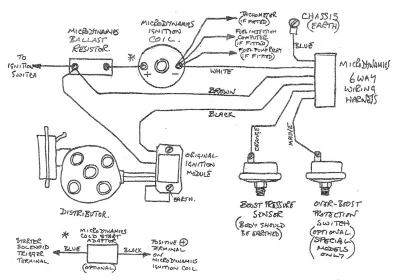
1. COIL MUST BE CHANGED TO A MICRODYNAMICS MACRO SPARK TYPE, 2. DO NOT MAKE ANY CONNECTION TO WIRING BETWEEN DISTRIBUTER & MODULE. 3. TACHOMETER AND FUEL INJECTION WIRING MUST BE CONNECTED AS SHOWN.
