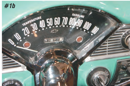
Photo #1a & 1b: The 1955-56 cars actually had a different instrument bezel between manual and automatic transmissions. On manual shift cars, the window for the indicator was not even cut out. Replacing the bezel can be fairly costly and cutting the window is all but impossible.
