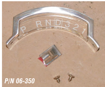
Photo #2: The new shift indicator anchors to the head of the steering column with two sheet metal screws while the pointer anchors to the shift collar with double sided tape. The indicator has a clear lens with a polished billet bezel and billet
