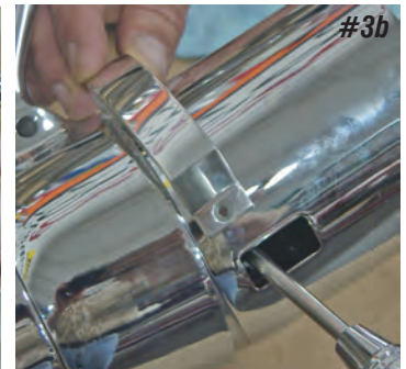
Photo #3a & 3b: With the column in the tilted position, locate the indicator on the steering column head at 12 o'clock. This will put the left hand edge of the billet bezel about 3/8" from the hole in the column for the tilt lever.
