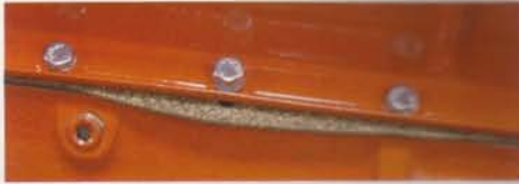
Photo #5: With the old-style gaskets and seals in place, the oil pan can be bolted to the
