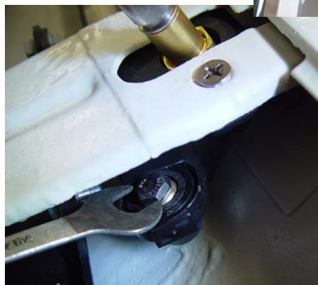
Photo ABO-10: Locate the driver side Pivot Shaft Lever under the driver side Intercostal.
