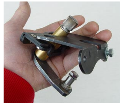
Photo ABO-3: Place the Body Bracket on top of the Pivot Shaft Assembly.
