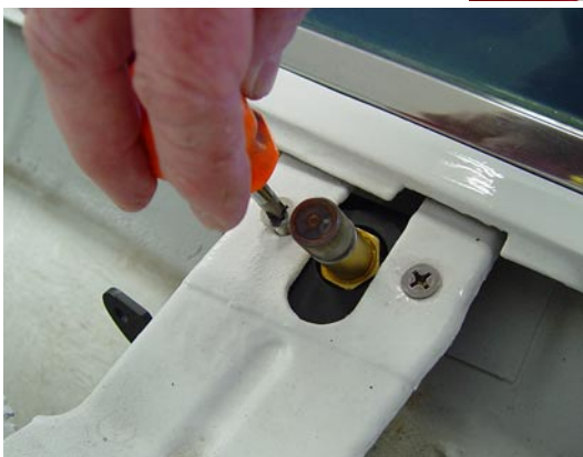
Photo ABO-4: Install the Body Bracket and Pivot Shaft Assembly under the left, driver side, intercoastal.
