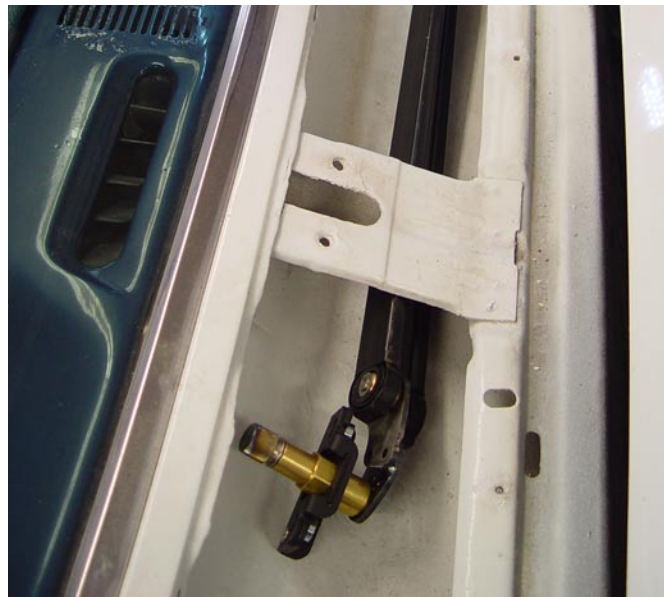
Photo ABO-9: Orient the Pivot Shaft head aft.
