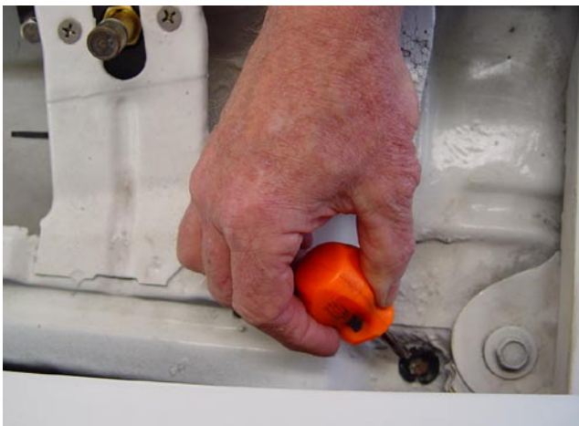
Photo ABO-5: Remove the OEM hole plug.
