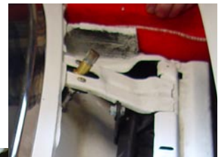
Photo ABO-10: Locate the driver side Pivot Shaft Lever under the driver side Intercostal.
