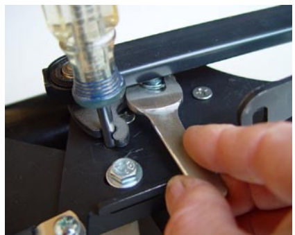
Photo ABO-11: Align the "Parking Features, Tighten the Spindle Nut. In this photo the unit is not installed to better show what is needed.
