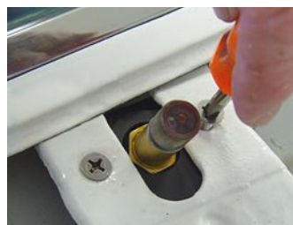
Photo ABO-9: Orient the Pivot Shaft head aft.
