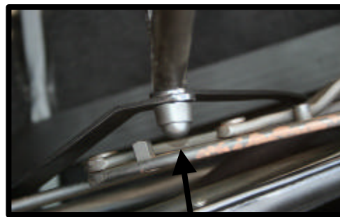
Fitting point of bracket with the bolt of persenning
