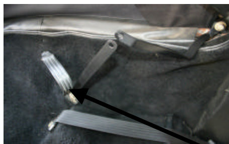
Fitting point of bracket with the bolt of persenning
