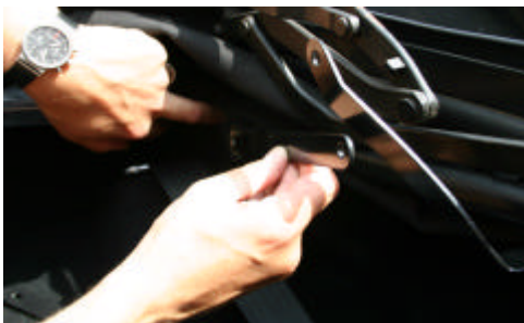
Fixingpoints for bracket Softtop has to hold in a open position for fitting of bracket
