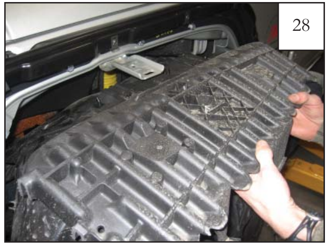
Replace factory inner structure/splash shield in fender as shown, sliding hole in structure over metal fender bracket.
