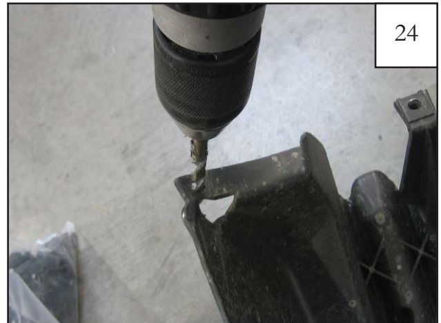
Drill one 5/16" hole in tab at forward area of splash shield as shown. The point of the drill should be approximately 5/16" down from top and 1/2" in from edge of tab.
