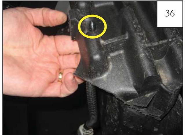
Reinstall Christmas tree clip in hole in factory Inner structure. Reconnect light cord to wire harness.
