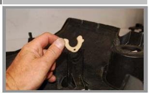
To re-install the engine cover, remove the white rubber clip from the underside of the engine cover, on the passenger side, next to the oil cap fill hole. Install the cover and re-install the oil cap. The oil cap and front driver side mounting pin will hold the cover into place. The heater hoses may need to be re-positioned to the left side of the passenger side fuel rail.
