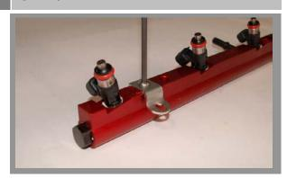
Install the supplied mounting brackets onto the bottom of the BBK Fuel Rails using supplied 1/4"-20 button head screws. Use the holes marked LS2.
