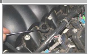
Use the four .300" tall black aluminum spacers under the mounting brackets, one per bracket, and install the assembled fuel rails into the intake manifold. Secure with the provided button head screws and washers. Give the rails a push down to seat the injectors into their bungs.
