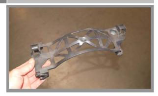
Remove the rear engine cover plastic mounting bracket. This will NOT be re-installed.
