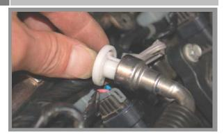
Using the 3/8" spring lock tool, remove the fuel feed line from the driver side rail.
