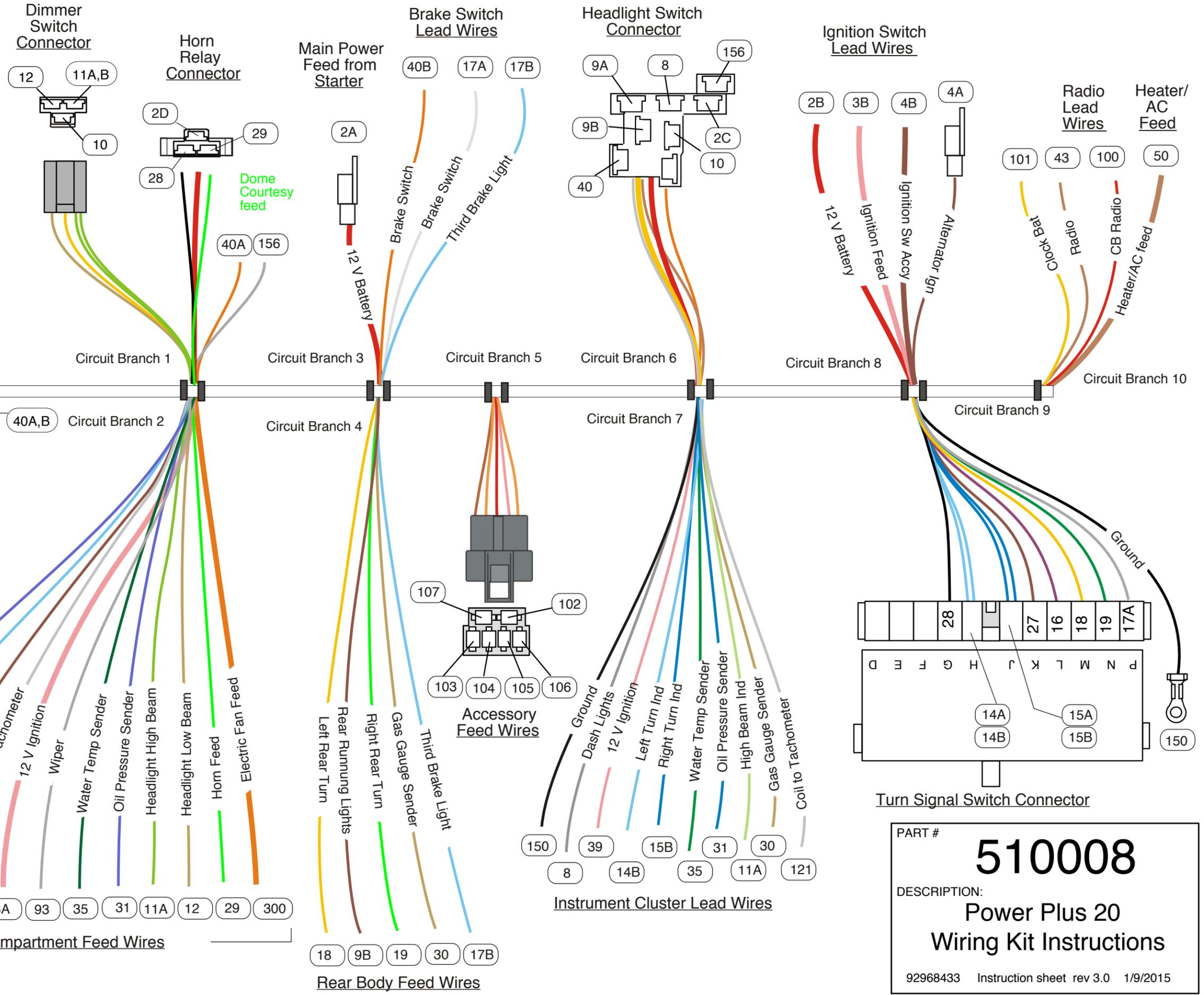
Engine Compartment Feed Wires: 15A, 14A, 9A, 121, 3A, 93, 35, 31, 11A, 12, 29, 300
