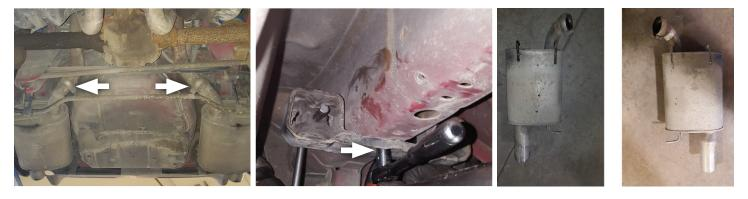
4. Transfer mounts from factory to FFX mufflers. Remove nuts from clamps, apply anti-seize compound to bolts and re-install nuts.
