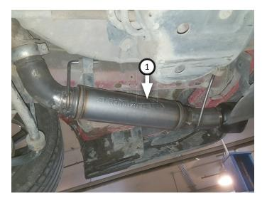
Place clamp (removed step 3) onto left muffler assembly (2) then connect it to left exhaust outlet. Insert wire hangers into isolators and tighten clamp just enough to allow for later adjustment.
