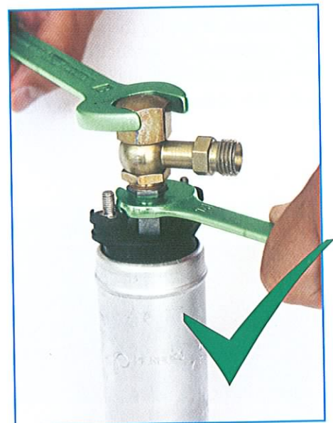
Fig. 71 Correct installation: The lower hexagonal bolt of the fuel pump must be locked in place
