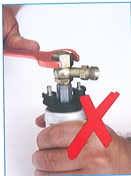
Fig. 70 Incorrect installation: Fastening without locking
