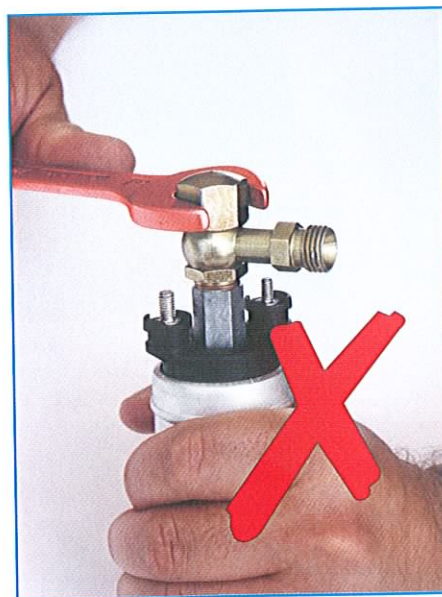
Fig. 70 Incorrect installation: Fastening without locking
