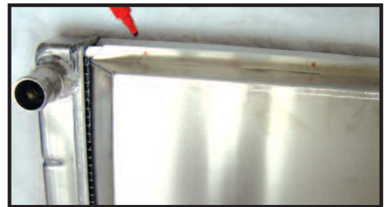
PHOTO 5: Marking outer flanges.
