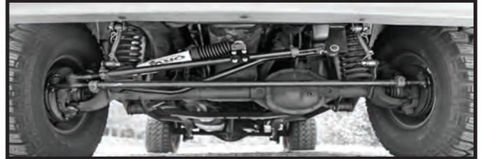
**Warning:** Steering system has been designed to work with most factory and aftermarket wheel-tire combinations. Some aftermarket and factory wheels with deep backspacing could make contact with passenger side cross over tie rod end at full LH steering lock. CHECK FITMENT OF WHEELS-TIRES PRIOR TO INSTALLATION.
