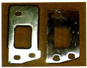
**Photo #5:** The rear edge of the stock hood latch plate will need to be trimmed 1/2" to clear the AC condensor. This can be done with a hack saw. If you want to dress your car up a bit, a new polished billet hood
