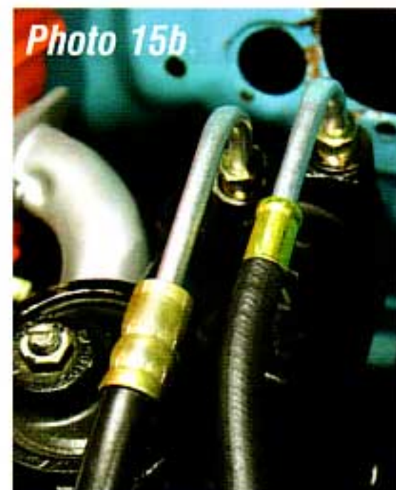
Photo #15a & 15b: The return hose P/N 53-31 connects to the barbed nipple on the back of the power steering pump with a hose clamp and the smaller port on the power steering box.
