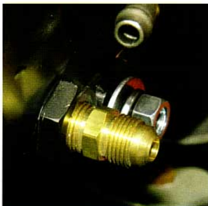
Photo #12: The pressure port on the rear of the power steering pump is a 3/8" female inverted flare fitting. A brass adapter is included with the power steering pressure hose P/N 53-32. The brass fitting allows the female end of the pressure hose to connect to the power steering pump.
