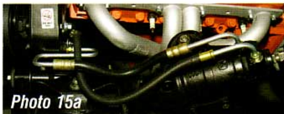
Photo #15a & 15b: The return hose P/N 53-31 connects to the barbed nipple on the back of the power steering pump with a hose clamp and the smaller port on the power steering box.
