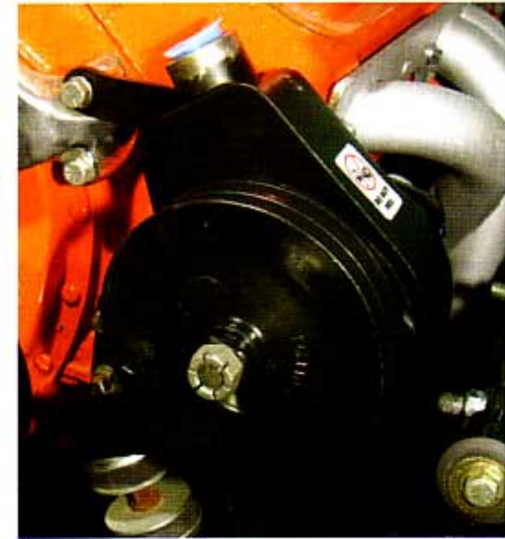
Photo #7: The double groove power steering pump pulley P/N 53-30 has a slotted keyway and is held to the pump with a 3/4" nut supplied with the power steering pump.
