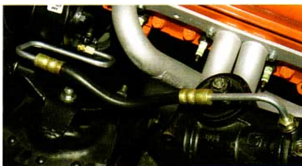
Photo #14: The male end of the pressure hose has an 3/8" inverted flare and screws into the larger of the 2 ports on the steering box.
