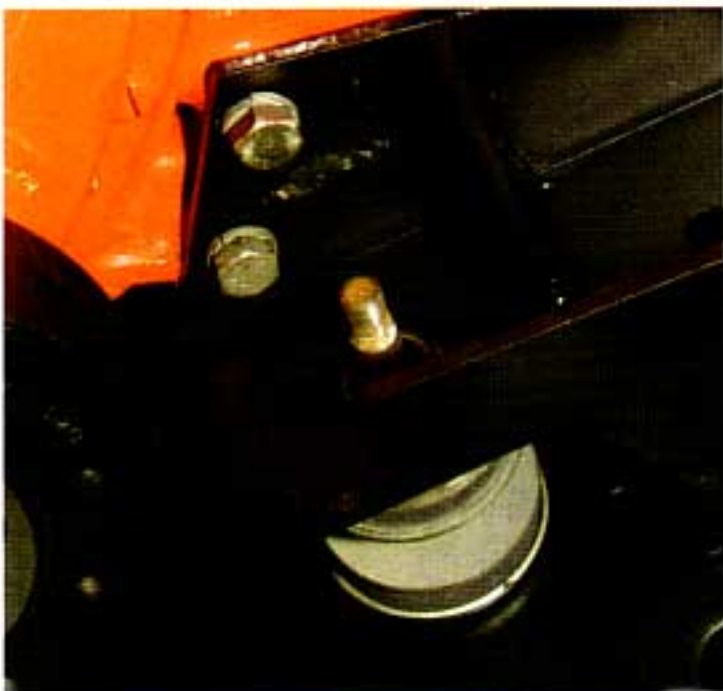
Photo #2a & 2b: The engine must be supported on the driver's side using a floor jack or engine hoist. Raise the driver's side of the engine so that there is no load on the left front engine mount. Remove the two 9/16" X 1" bolts and lock washers and the angle mount.
