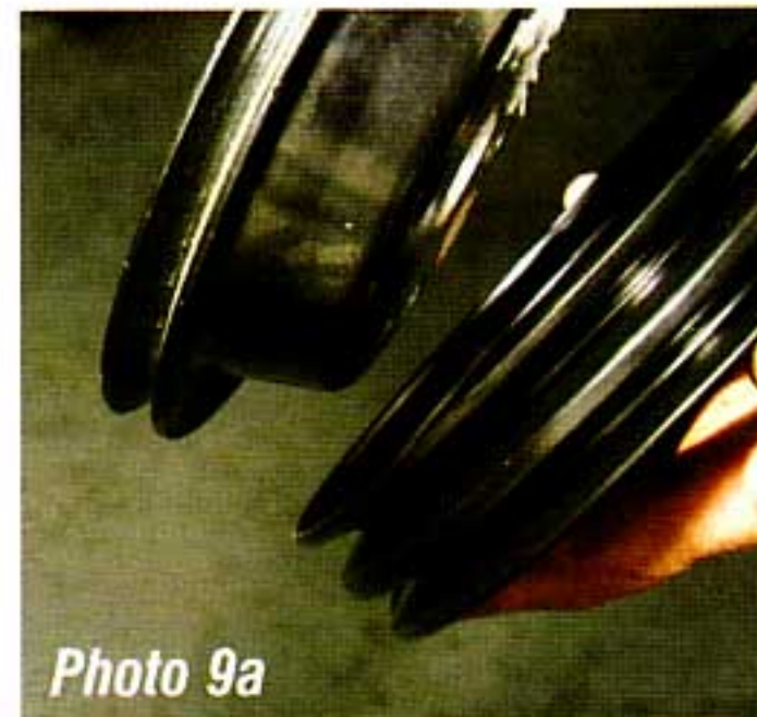
Photo #9a & 9b: The first groove (closest to the timing cover) on the crankshaft pulley P/N 51-03 drives the water pump and generator or alternator belt. The second groove drives the water pump and air conditioning compressor. The third groove pulley P/N 53-34 drives the power steering pump. The pulleys are held to the harmonic balancer with three 3/8" fine thread bolts.
