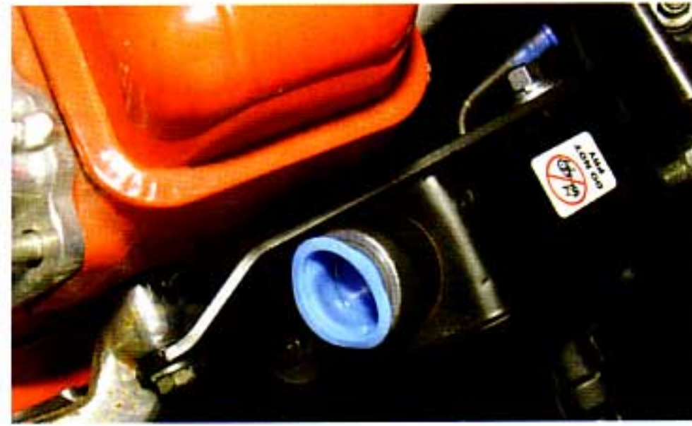
Photo #6: The power steering pump adjusting arm bolts to the top of the water pump using the original bolt. The slotted end of the adjusting
