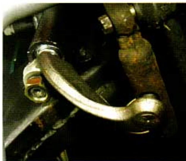
Photo #16: When installing a 605 or 670 power steering box, original non-power steering linkage must be used. The original pitman arm fits directly on to the 670 pitman shaft.
