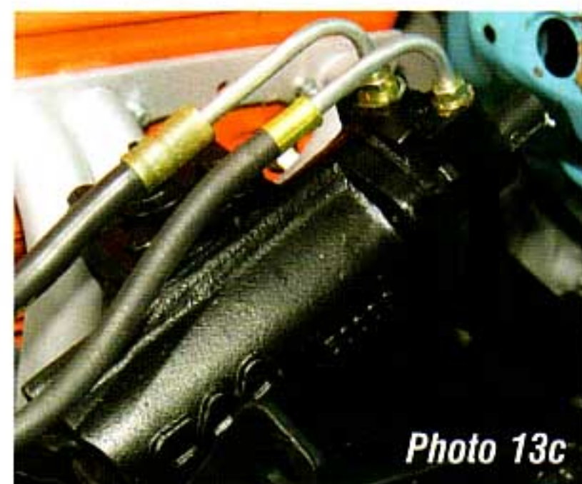
Photo #13a, 13b & 13c: The 670 box bolts to the frame using the stock steering box bolts. The input shaft is the same size and location as the 605 power steering box and uses the same pressure and return hoses as an inverted flare type 605 steering box.
