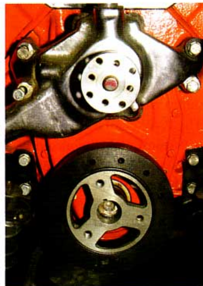
Photo #8: If your engine has a harmonic balancer with the lower crankshaft pulley riveted on, it must be replaced with a balancer that will accept bolt-on crankshaft pulleys. P/N 18-35 is a 6-3/4" diameter small block harmonic balancer that will work with the front engine mounts and any internally balanced small block Chevy.
