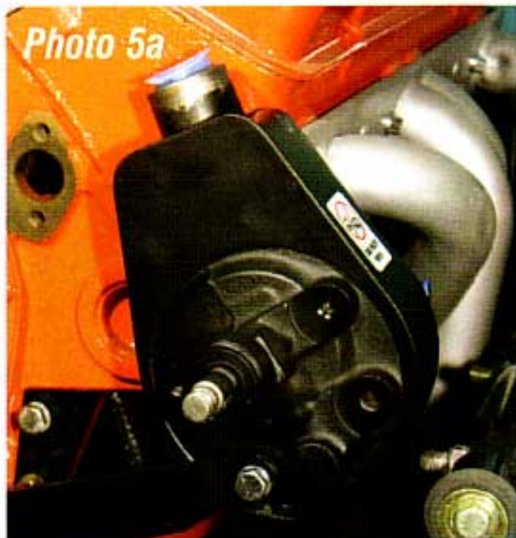
Photo #5a & 5b: The power steering pump P/N 53-28 mounts to the bracket using a 9/16" X 1" bolt and lock washer on the front and a 9/16" nut, lock washer and flat washer on the rear stud of the power steering pump.
