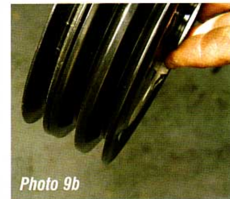
Photo #9a & 9b: The first groove (closest to the timing cover) on the crankshaft pulley P/N 51-03 drives the water pump and generator or alternator belt. The second groove drives the water pump and air conditioning compressor. The third groove pulley P/N 53-34 drives the power steering pump. The pulleys are held to the harmonic balancer with three 3/8" fine thread bolts.
