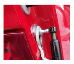
Install the narrow end of the shock on the ball mount.
