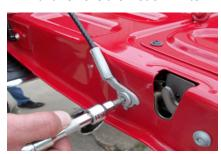
The flat retaining nut must be taken off to remove the limiter.
