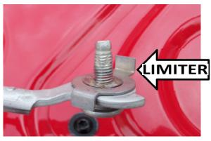
Once the limiter is removed, reinstall the cable mount to the tailgate.
