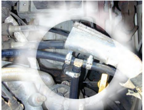
1. Connect one end of the main fuel feed line to the fuel Tee connector and securely tighten.
