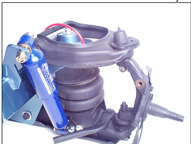
Mustang II with OEM lower a-arm
