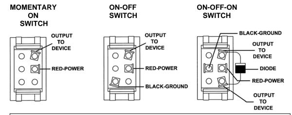
DIODE INSTALLATION: With diode stripe on top (as shown) it will send power out the bottom and top output wires when the top of the switch is pushed, but it will only send power out the top output wire when the bottom side of the switch is pushed. It will be opposite if the diode is reversed.
