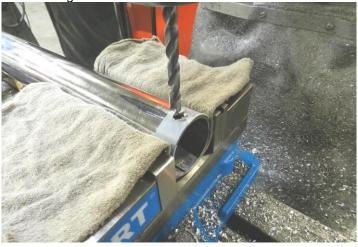
5. Now do the same with the bottom tube using the paper strip labeled 206250 that has the holes centered. The alignment of this tube will not matter because it is the same all around.
