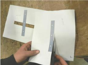
2. The two templates are different. The one has the three holes in the center and the other has the three holes offset to one side. Use the offset one labeled 206230 for the top half, the upper bell side, of the column. The holes will go closest to the top of the column as pictured. Tape the strip with the slit in the direction where you want the electric motor to point. We aligned the slit with the top of the column so the motor will point straight up.
