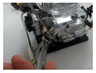
Once the chrome flare nuts have been snugged up by hand, the installer should then use two properly sized wrenches and apply the final torque to this connection. By holding the brass fuel bowl fitting with one wrench, and then applying torque to the chrome flare nut with another wrench the installer will be able to stop any damage from happening to the gasket when applying torque to the chrome flare nut.
