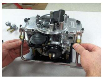
It is suggested that the installer start threading both chrome flare nuts into the brass fuel bowl fittings at the same time. This will insure that both ends of the chrome fuel line will be centered in their respective brass flare and will tighten up evenly.
